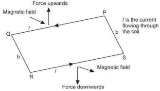
Due to this radial field, the sides *QR* and *SP* are always parallel to the *B*-field (magnetic field) and experience no force. The sides *PQ* and *RS* are always parallel to the *B*-field and experience force and due to this, torque is produced.
